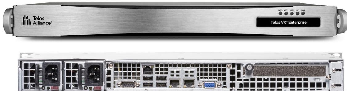
VX Enterprise 1RU rack-mount device is the heart of the system. It provides all the call control and audio processing needed for the system, and supports up to 120 active calls on-air simultaneously. Its two Gigabit Ethernet ports provide a cost-effective interface to both telephone lines and studio audio via proven Livewire AoIP. VX Enterprise is Web-based, so remote control and configuration are a snap — engineers can work with it from any place they can get online.
